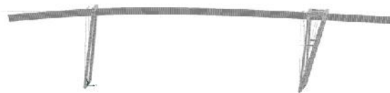
Figure 7. Deformation of cranes from the force at the end of the elastic leg
