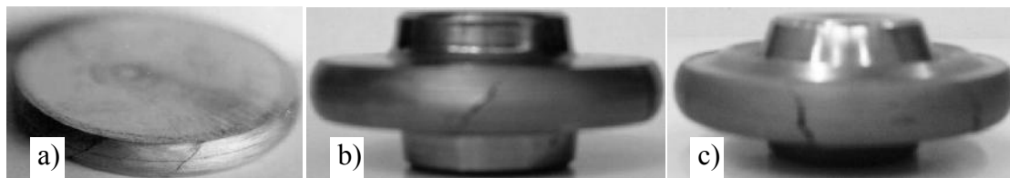
Figure 3. Samples after destruction: a) Flat plates, b) Hollow plates, c) Hollow plates with concentric channels
