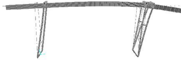
Figure 6. Deformation of cranes from the force at the end of the rigid legs
