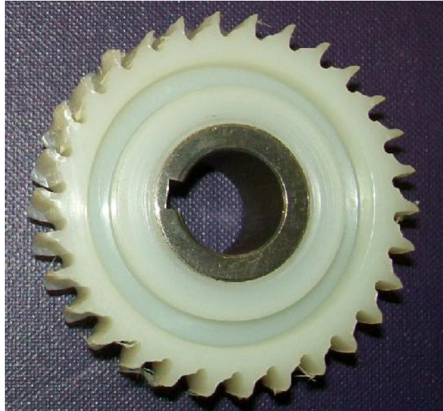
Figure 1. A nylon gear having failed by gross wear and thermal melting
