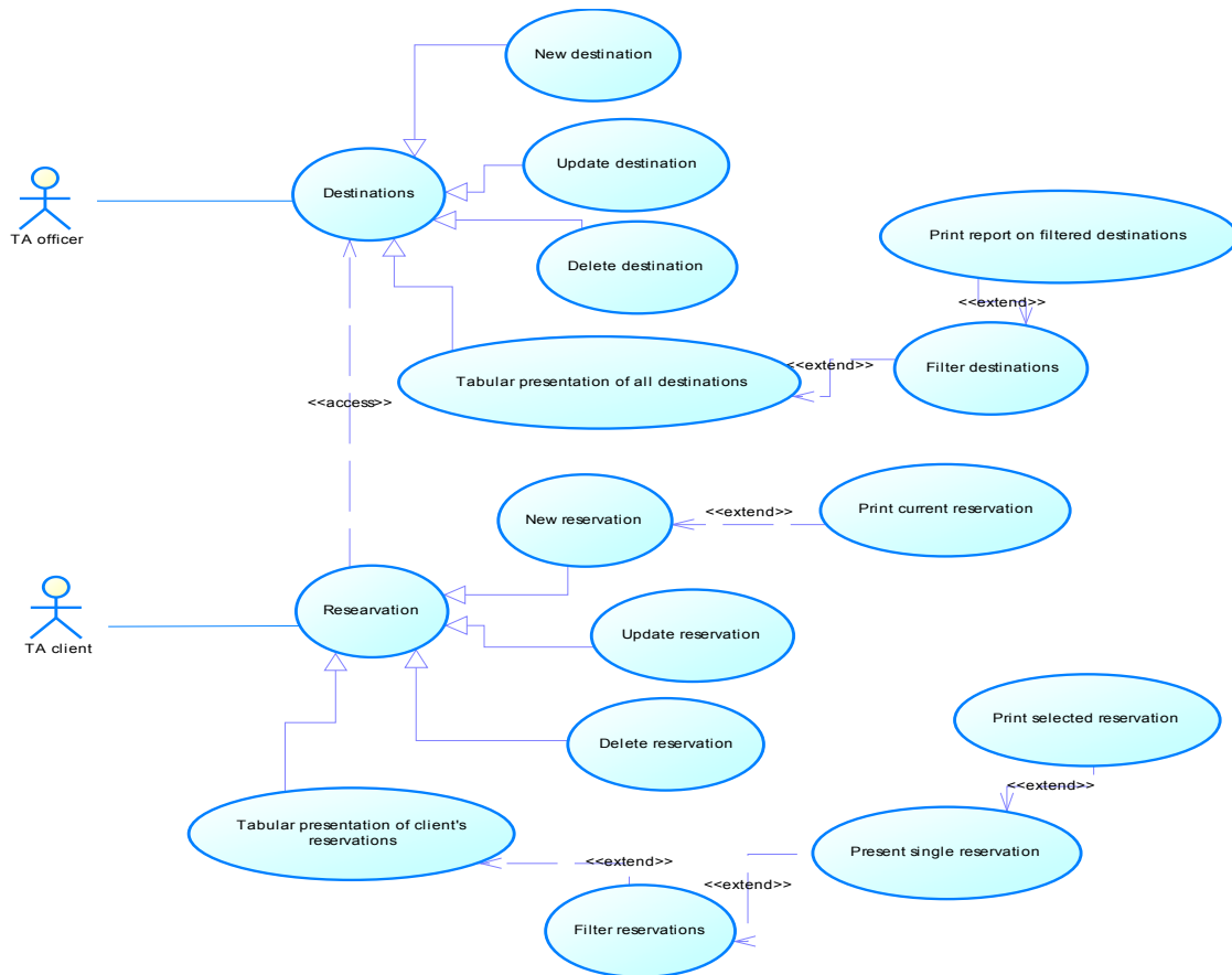
Figure 8. Use case diagram for example of tourism agency web application software project
