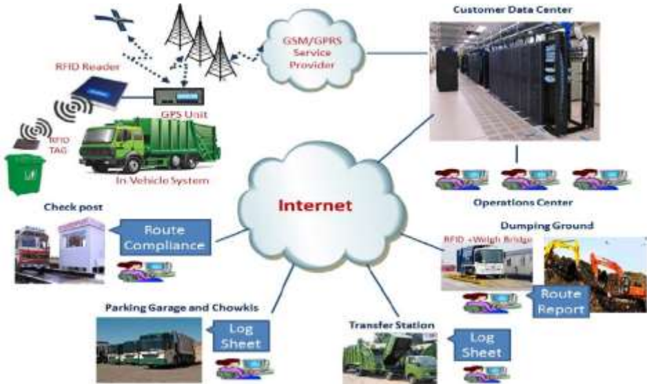
Fig. 1. Architecture of the Solid Waste Management System
