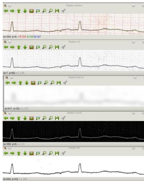
Fig.3. Algorithm stages of time series recognition
