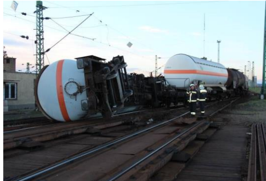
Fig. 2. The overturned tank car filled with liquefied isobutene at the marshalling yard of Miskolc [9]
