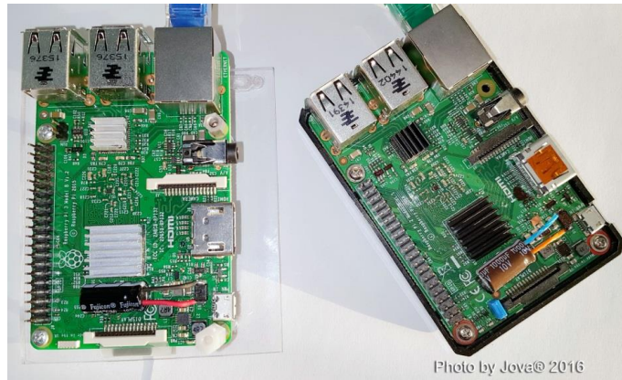
Figure 1. Raspberry Pi 3 and Pi 2 with the installed coolers and modified voltage level regulator
