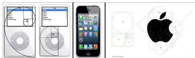
Fig. 6. Golden section in the design of the iPad, iPhone5 and Apple logo factory
