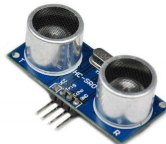
Figure 2. HC - SR04 Ultrasonic sensor [11]
