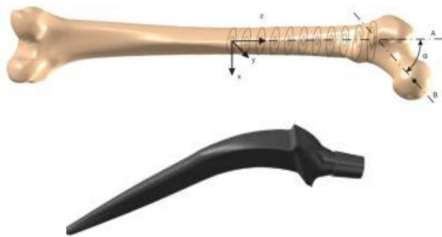
Figure 7. Computer model of the femur (up) and the endoprosthesis body (down) [5]
