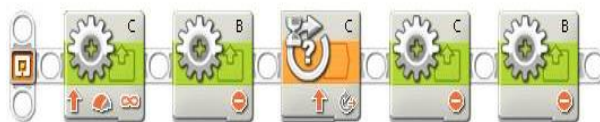
Figure 2. Sample from the NXT program for a measured turn. Motor C goes forward, motor B is stopped and the sensor is set to wait 720 degrees. After the turn, both motors are stopped.
