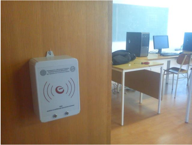
Figure 3. A prototype of the RFID reader mounted at computer laboratory entrance
