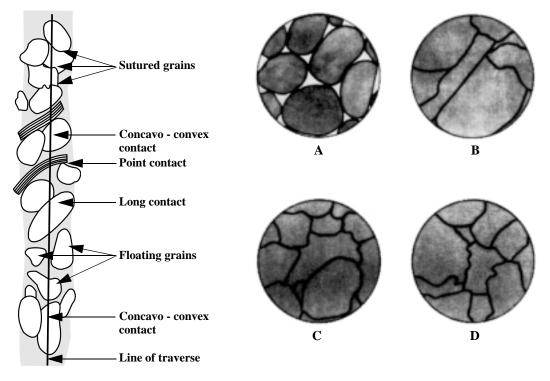
Figure 1-3 Grain Contact Terminology: A) point contact, B) long contact, C) concavo-convex, D) sutured
