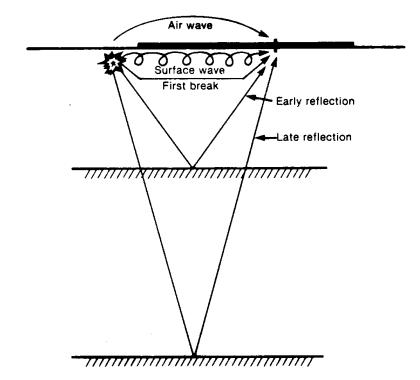
Figure 6-7 Types of Reflections from a Seismic Shot
