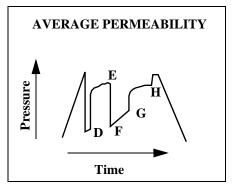
On this chart, the shape of the two shut-in curves (DE and GH), the rate of shut-in pressure buildup, and the indicated influx of fluid during the final flow (line GF) suggests a zone of average permeability.
