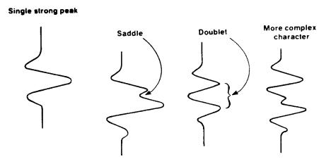
Figure 6-9 Character of Seismic Wiggles
