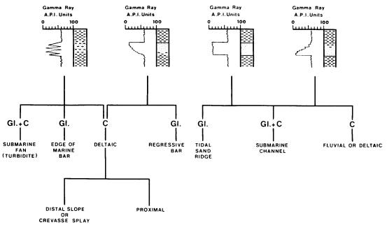
Characteristic log motifs. From left to right: thinly interbedded sand & shale: an upward coarsening profile with an abrupt upper sand/shale contact: a uniform sand with abrupt upper & lower contacts & furthest right, an upward fining sand: shale sequence with an abrupt base.
