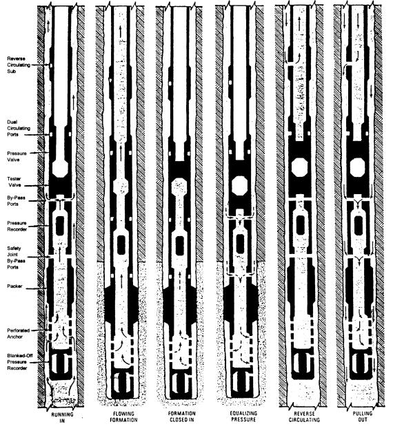
Figure 8-2 TESTING - Fluid Passage Diagram (from Halliburton Services)
