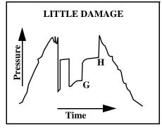
By comparison, this chart shows relatively little damage to the reservoir. The radius of curve GH is longer with a slope and the differential pressure is not as great between final flow (G) and final shut-in (H).
