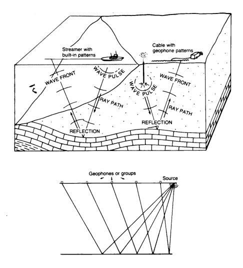
Figure 6-1 Generation of Seismic Reflections
