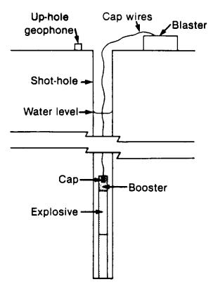
Figure 6-4 Schematic of an Onshore Shot-Hole
