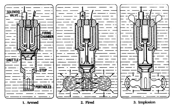
Figure 6-6 Water Gun Operation
