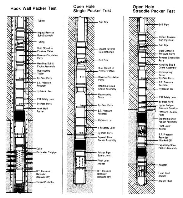
Figure 8-1 Three Basic DST Assemblies (from Halliburton Services)
