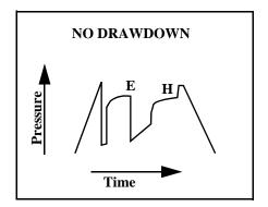
However, where the difference between the initial shut-in pressure (E) and the final shut-in pressure (H) is less than two percent, as it is here, the chart would suggest not only high permeability but also a potentially commercial reservoir.
