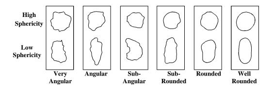
Figure 1-2 Grain Shape based on roundness and sphericity
