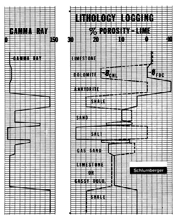
Figure 5-6 Lithology Determination Using GR and N-D Log
