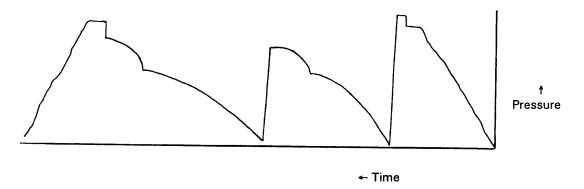
Figure 8-4 Double Shut-in Pressure Record
