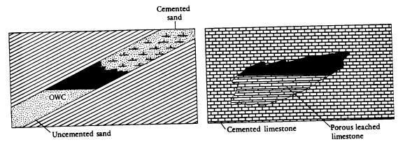
Figure 4-7 Stratigraphic Traps Resulting From Changes In Their Depositional Environment
