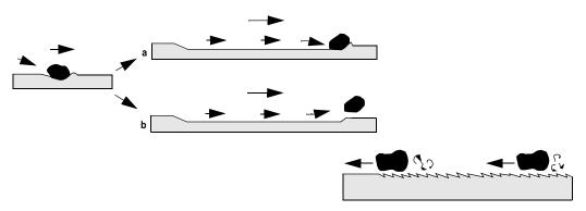
Figure 2-9 The development of a groove mark caused by a moving object.
