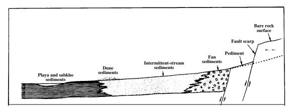
Figure 3-1 Map View (A) and Cross-Section (B) of Alluvial Fan Environment
