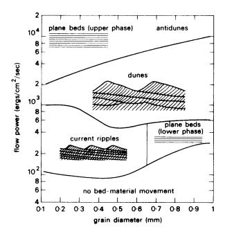
Figure 2-6 Relationship between flow velocity, grain size and bed form.
