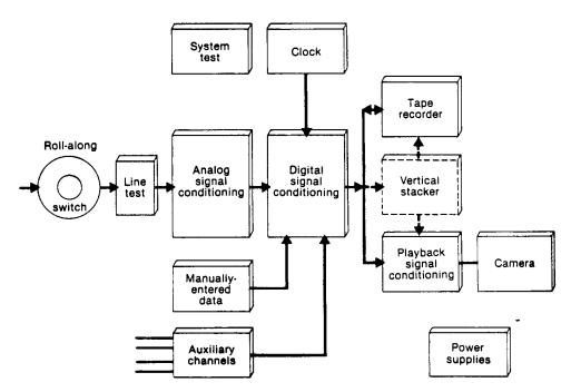
Figure 6-5 Seismic Recording Instrument Layout
