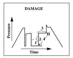
With some exceptions, a damaged zone will be indicated by the configuration of the shut-in curve (GH). Specific indicators are a very sharp rise after the final flow (1), a short curve radius (2), a reasonably flat slope (3), and a high differential pressure between the final flow and final shut-in (4).
