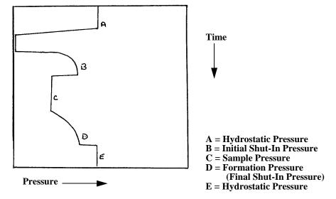
Figure 8-7: Typical Medium Permeability Pressure Record.
