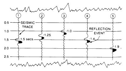
Figure 6-3 Generation of Seismic Traces
