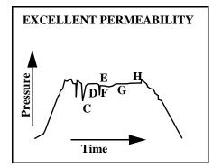
This chart, on the other hand, suggests a zone with high permeability. The shut-in curves (DE and GH) were developed faster, and the flow curves (CD and FG) indicate a high rate of fluid entry to the test tool.
