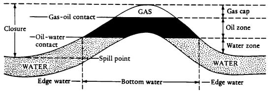
Figure 4-3 Cross-section Of A Simple Anticlinal Trap
