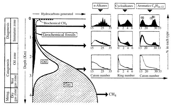
Figure 7-3 The Oil Window, and General Scheme of Hydrocarbons Produced (Modified after Taoist et al., 1974)
