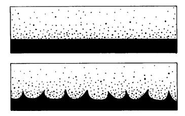
Figure 2-8 Load structures developing on the lower surface of a sand layer resting on a clay layer.
