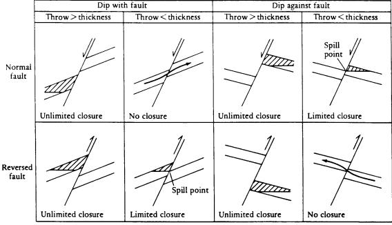
Assumption: Shale against sand is sealing. Sand against sand is nonsealing.
